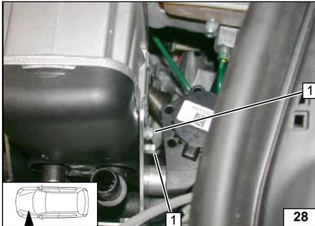
1 Tighten 5x13 self-tapping screws [2x]
