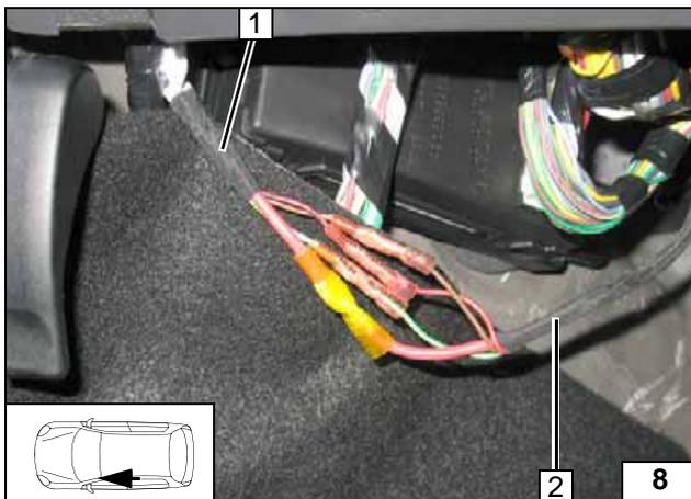
Connect same colour wires of the wiring harness of the passenger compartment fuse holder 1 to those of the heater wiring harness 2 as shown in wiring diagram.
