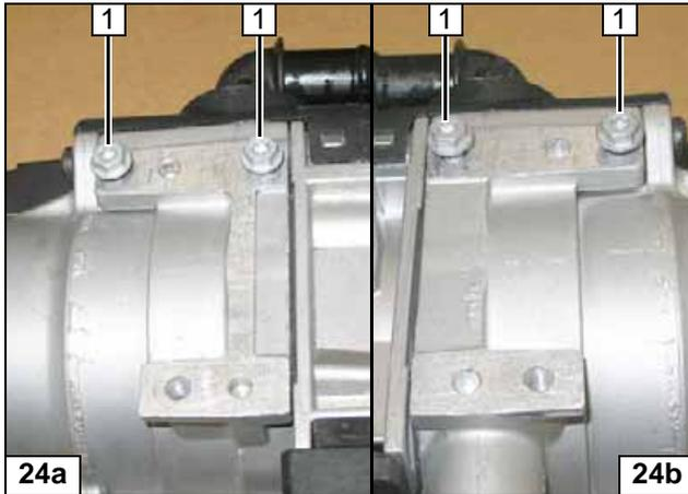
Tap thread with 5x13 self-tapping bolts 1 [4x] and mount loosely (max. 3 thread turns).
