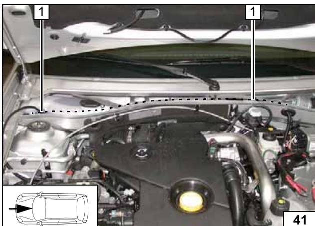
Route fuel line and wiring harness of metering pump to coolant reservoir on the right vehicle side.
