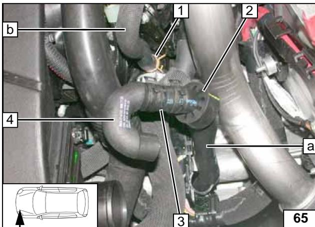
Expansion tank removed for better display. Install hose of expansion tank supply line **b** as shown. Slide black (sw) rubber isolator **2** on to hose of expansion tank supply line **a**.
