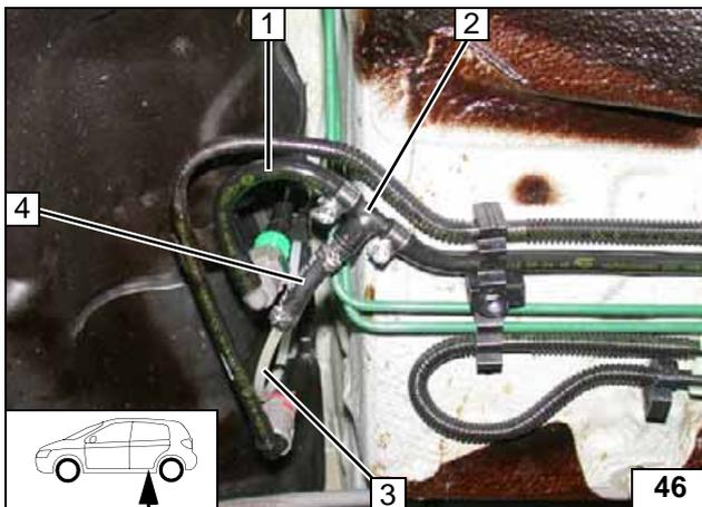
Cut off fuel supply line 1 as shown.
