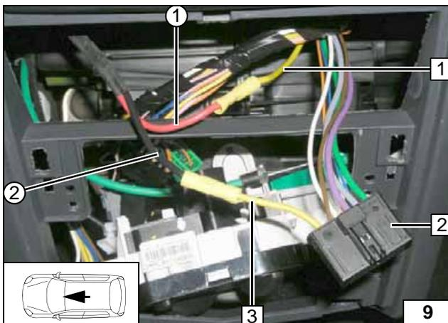
Connection to 6-pin connector B 2 from fan switch.
