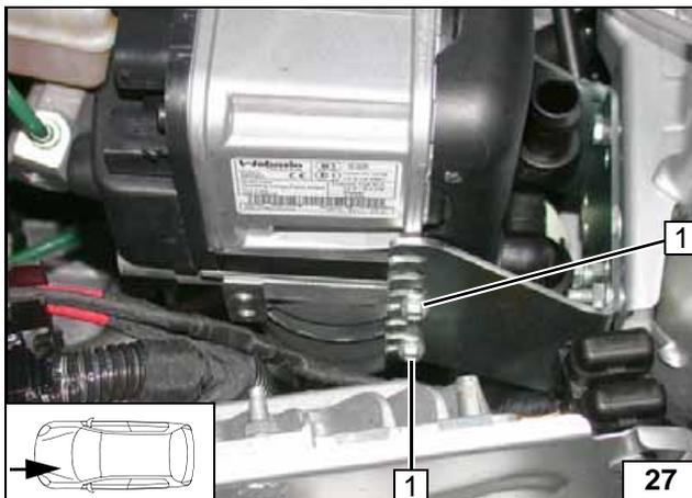
1 Tighten 5x13 self-tapping screws [2x]
