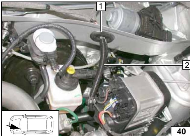
Route fuel line and wiring harness of metering pump in corrugated tube 2 to the coolant reservoir.
