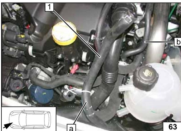
Cut off hose of supply line to expansion tank **a** at the marking. Remove hose of expansion tank supply line **b**. Spring clips will be reused.
