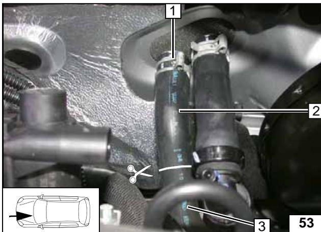
Cut hose of engine outlet / heat exchanger inlet **3** at the marking.
