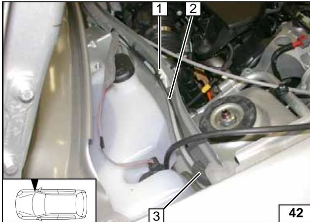
Slide on fabric protective hose 3 on fuel line and wiring harness of metering pump 2 and position in original vehicle pass through.
