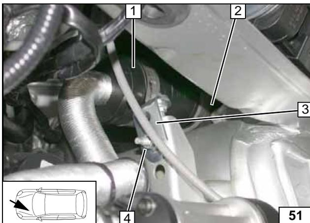
Paste insulation strip 2 as flap protection on silencer 1.
