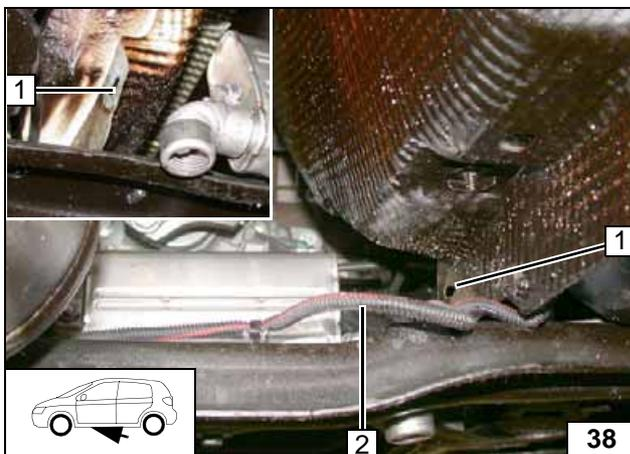
Detach original vehicle wiring harness **2** at position **1** and tie back with cable tie. Ensure sufficient distance from neighbouring components.
