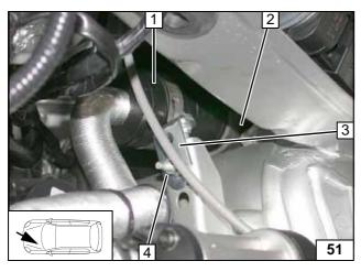
Paste insulation strip **2** as flap protection on silencer **1**.
