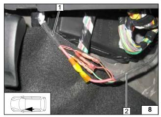
Connect same colour wires of the wiring harness of the passenger compartment fuse holder 1 to those of the heater wiring harness 2 as shown in wiring diagram.
