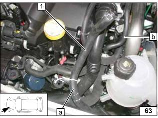
Cut off hose of supply line to expansion tank **a** at the marking. Remove hose of expansion tank supply line **b**. Spring clips will be reused.
