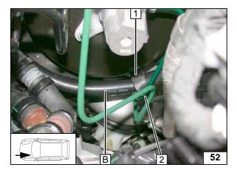
Route hose **B** to cutting point. Align black (sw) rubber isolator **1** and fasten with cable tie **2** to the original vehicle line.
