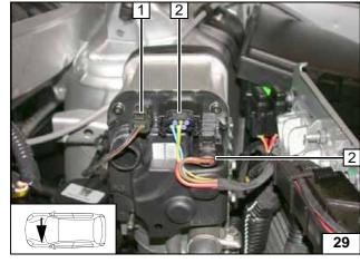
1 Wiring harness of circulating pump2 Wiring harness of heater [2x]
