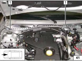
Route fuel line and wiring harness of metering pump to coolant reservoir on the right vehicle side.
