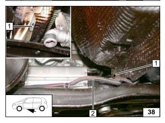
Detach original vehicle wiring harness **2** at position **1** and tie back with cable tie. Ensure sufficient distance from neighbouring components.
