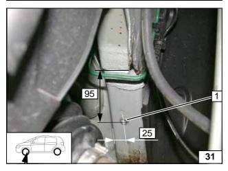
1 9.1mm dia. hole, rivet nut
