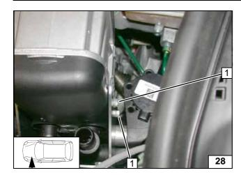
1 Tighten 5x13 self-tapping screws [2x]
