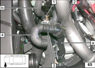
Expansion tank removed for better display. Install hose of expansion tank supply line **b** as shown. Slide black (sw) rubber isolator **2** on to hose of expansion tank supply line **a**.
