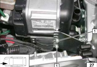
1 Tighten 5x13 self-tapping screws [2x]
