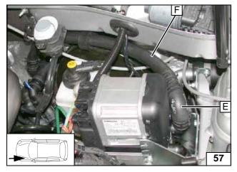
Align hoses. Ensure sufficient distance from neighbouring components.
