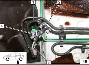
Cut off fuel supply line 1 as shown.
