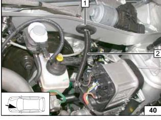
Route fuel line and wiring harness of metering pump in corrugated tube **2** to the coolant reservoir.
