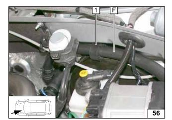
Slide black (sw) rubber isolator **1** on to hose **F** and align.
