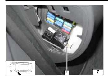
Insert fuse holder of passenger compartment into the recess, tighten bolt 1.
