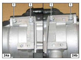
Tap thread with 5x13 self-tapping bolts **1** [4x] and mount loosely (max. 3 thread turns).
