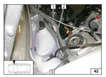
Slide on fabric protective hose **3** on fuel line and wiring harness of metering pump **2** and position in original vehicle pass through.
