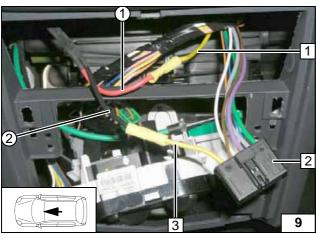
Connection to 6-pin connector B **2** from fan switch.
