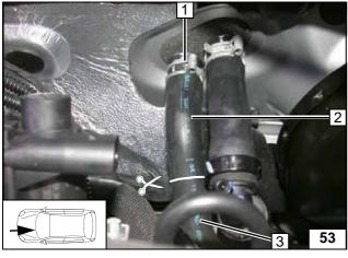
Cut hose of engine outlet / heat exchanger inlet **3** at the marking.
